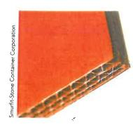
In doublewall or triplewall, varied flute profiles provide advantages over flutes of the same size that are perfectly aligned.
